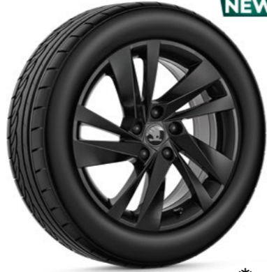
Nevis light-alloy wheel black metallic 6.5J x 17" ET46 for 205/55 R17 5E3 071 497J FL8 5E3 071 497AB FL8*
