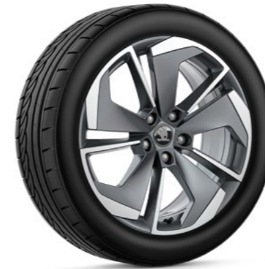
Comet light-alloy wheel anthracite metallic brushed 7.5J x 18" ET48 for 225/45 R18 5E3 071 498A HA7 5E3 071 498AL HA7*
