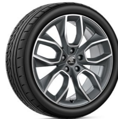
Manaslu light-alloy wheel anthracite metallic brushed 7.5J x 19" ET48 for 225/40 R19 5E3 071 499H HA7 5E3 071 499AG HA7*
