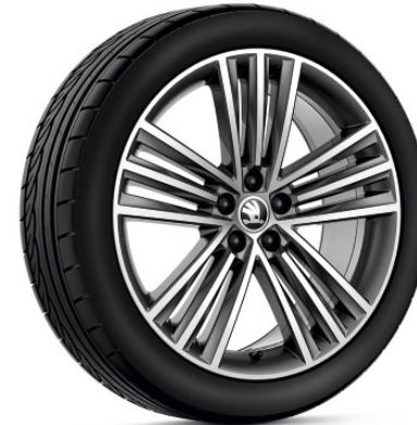
SIRIUS light-alloy wheel 7.0J x 18" ET39 for 215/45 R18 654 071 498F HA7 | anthracite metallic, brushed
