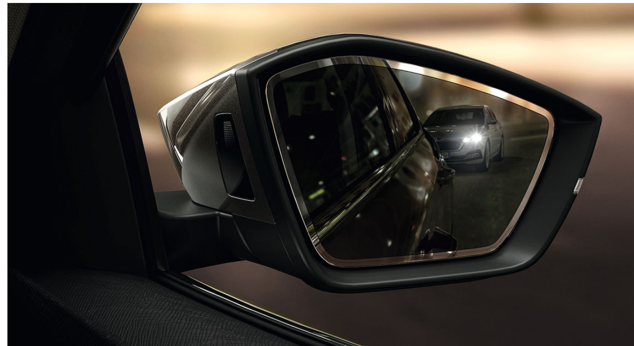
Auto dimming passenger mirror 658 072 538 | for LHD 658 072 538A | for LHD with Side View Assist The dimming function prevents glare from the car behind you.
