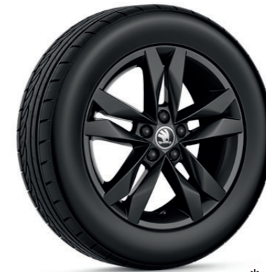
Canis light-alloy wheel black metallic 6J x 16" ET45 for 195/55 R16 6VE 071 496E FL8 6VA 071 496E FL8*
