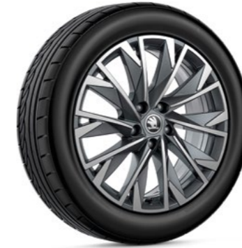
Hydrus light-alloy wheel anthracite metallic brushed 7.0J × 18" ET45 for 215/50 R18 (4×2), 225/50 R18 (4×4) 57A 071 498P HA7 57A 071 498AE HA7*
